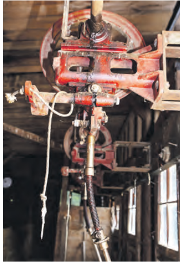
Mechanical shearing machines were installed in the early 1900s, and were originally powered by a steam tractor. PHOTO: CLAIRE INKSON
