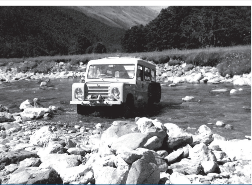
The Trekka had a New Zealand-designed and made body, on a kit-set Skoda chassis PHOTO SUPPLIED
